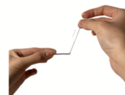
7) Place the capillary on the inlet of the test strip until the whole T channel is filled.
